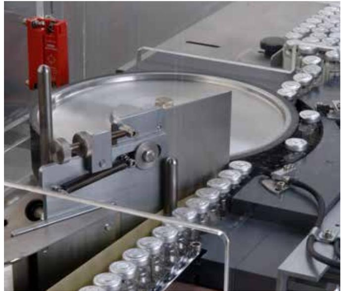
Some labelling systems offer an alternative, more efficient approach by allowing you to change over entire fitments in one go, which is certainly faster and less prone to error. The changeable fitment could be a starwheel, an entire feeding system, or just the guidance for the container. This is certainly better than adjusting all the machine settings individually, but it's not an overly sophisticated solution and it still takes time and skill.
